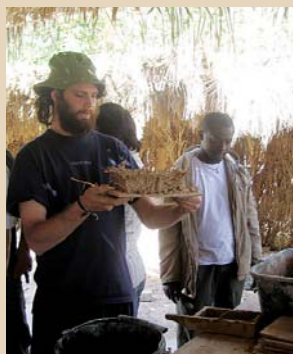
Seminar participants Ariel (a Venezuelan-Israeli gardener) and Frederick (an agro-engineer from Cameroon) produce sun-dried bricks. The same recipe the Children of Israel used to make mud bricks while in Egypt is applied today in the fabrication of carbon neutral walls, modern furniture, and pizza ovens.
